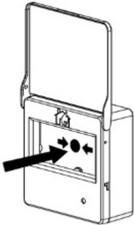
To press the button, it is necessary to lift the transparent protective cover, and press on the white sheet until it interlocks, a yellow indicator will appear at the bottom. The manual button will go into alarm status by activating the red LED continuously.
